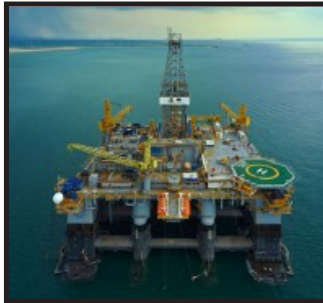
Deepwater Moored Semisubmersible
